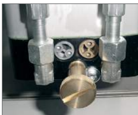
By pass valves
