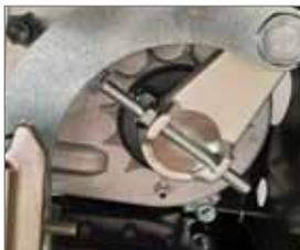
Adjustable mechanical stop in opening and closing
