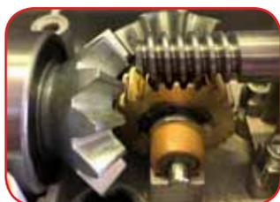
Metal gear drive with reinforced screw supported by ball bearings for maximum strength.
